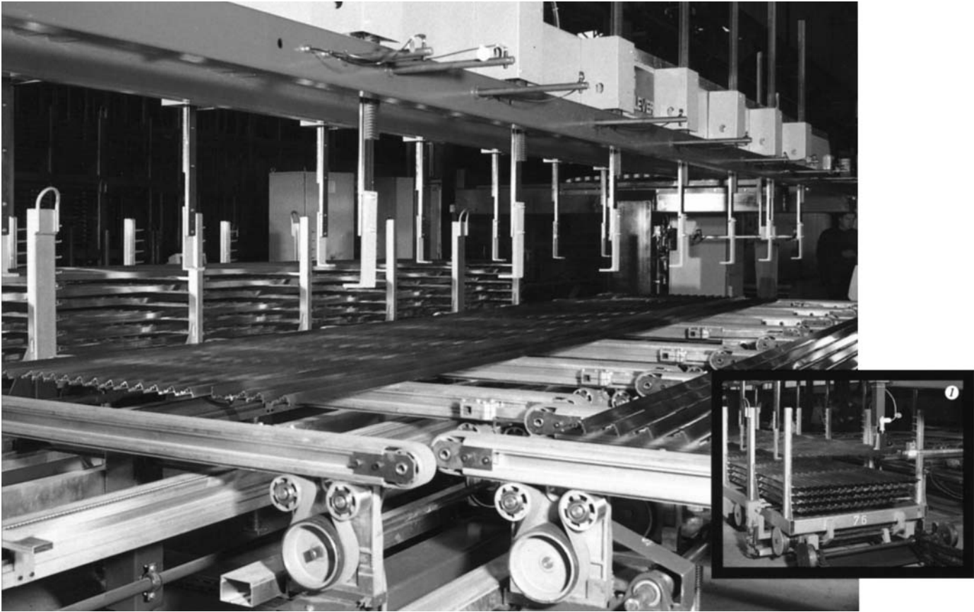
Fig. 32 Automatic section stacker. (1) Section stacker depositing in section basket. Source: SMS Engineering Inc.
