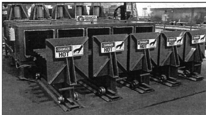
Fig. 25 Multicompartment die oven. Source: Granco Clark
