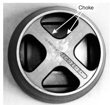
Fig. 20 Choke in a mandrel with equal bridge thickness of a single-hole hollow die. Source: Florida Extruder International, Inc.
