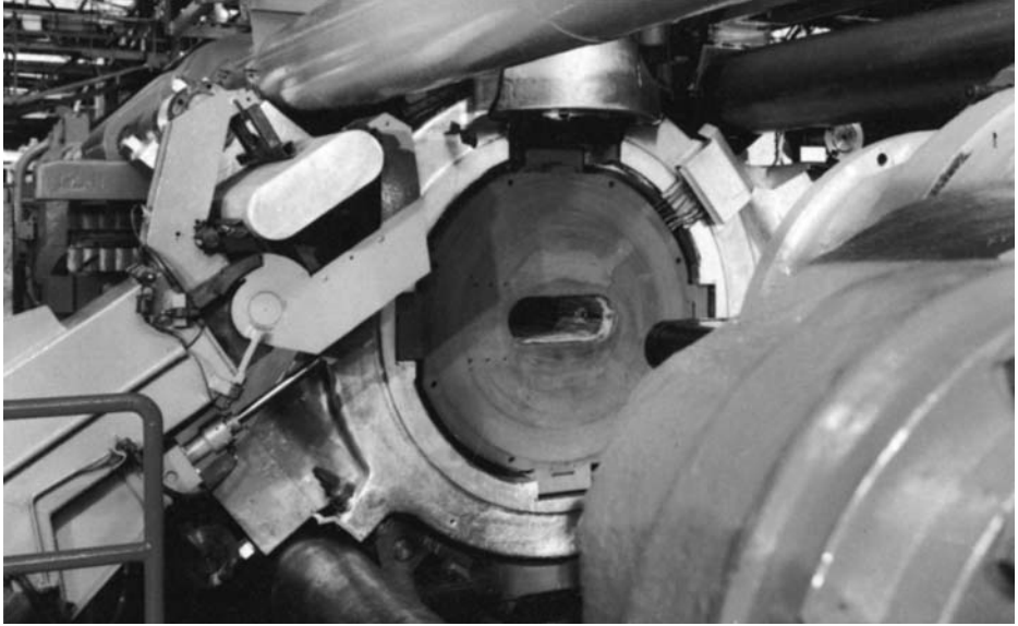
Fig. 11 Rectangular container with stem and billet loader. Source: Edelstahlwerke Buderus AG
