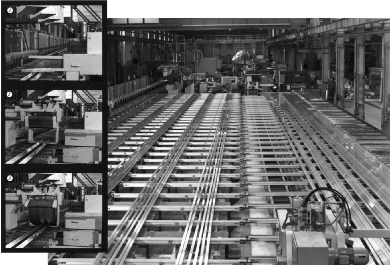
Fig. 28 Runout equipment showing hot saw and puller clamp. (1) Hot-shaping saw. (2) Puller with clamping blades opened. (3) Puller with sections gripped. Source: SMS Engineering Inc.
